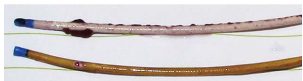
FIGURE 4. This figure shows the status of fibrin deposition on the catheter material after being exposed to blood for 60 min and then stained with hematoxylin. The control catheter is in the top part of the picture while the BIP catheter is placed on bottom.
